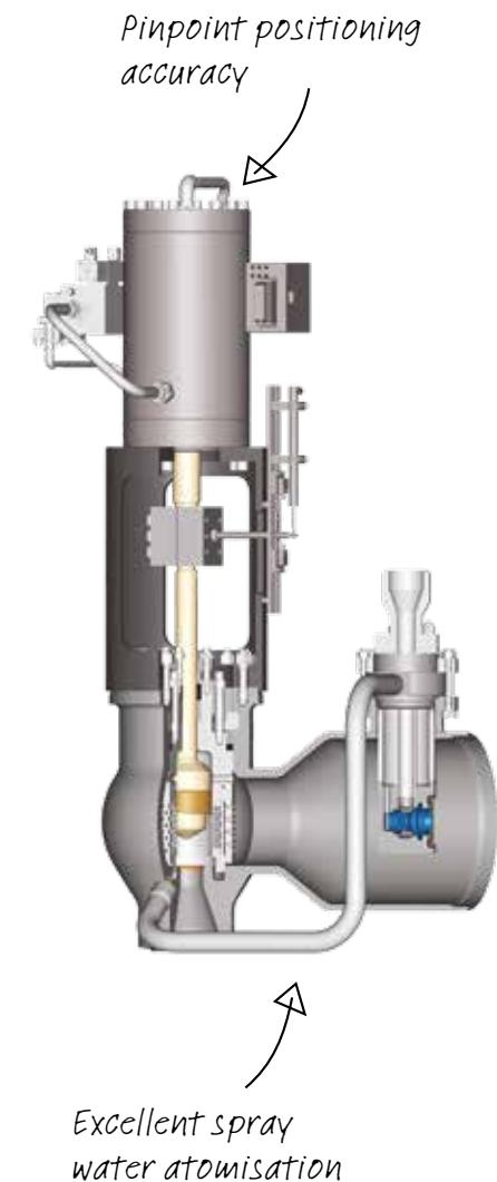
The trip signal is generated by a triple redundant safety cabinet. The entire system then meets the stringent DIN EN ISO 4126 – part 5 standards (formerly known as TRD 421) as a controlled safety pressure relief system (CSPRS).
